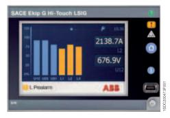
On the front of the trip unit there are also two LEDs: a pre-alarm LED (square yellow LED) and an alarm LED (red triangular LED); a message on the display always accompanies the flashing of the LEDs for clear identification of the type of event. The list of all the alarms active at that moment can be viewed by simply touching the display on the white strip in the bottom left of the alarms zone.
