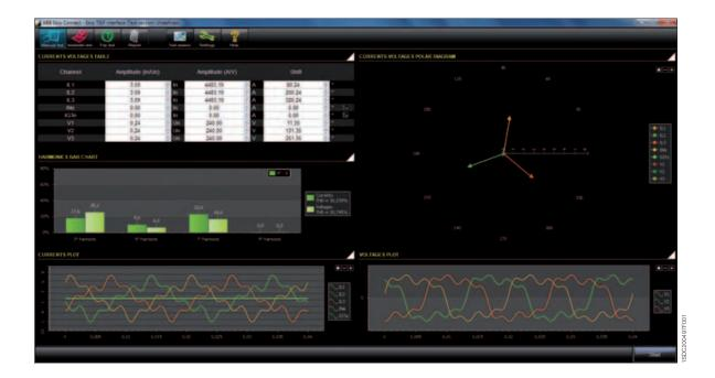
The software creates and stores all reports, keeping a record of the tests carried out and essential information such as the operator name, date, serial number of the circuit-breaker, type of test and the result.
