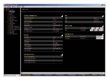
Ekip Connect automatically scans the RS-485 bus, detects all the devices connected and checks their configuration, checking all the possible address, parity and baud rate combinations. A simple click over SCAN will highlight:
