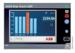
Alternatively, bar graphs that show the currents of the three phases and of neutral on a 0-125% In scale in addition to the numeric value of the most loaded phase can be selected as the default page. The bar graphs are yellow in the event of a pre-alarm and red in the event of an overload to enable an irregular condition to be identified immediately.
